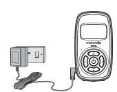
Insert the DC plug of the power adapter into the DC jack on the side of the parent unit.
