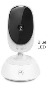
The blue LED on the camera is to indicate the linking and pairing status. This can also be seen from the parent unit.
