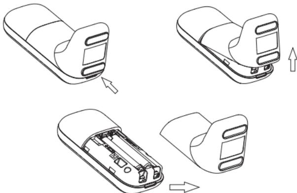
2. Insert the battery cells (not supplied). Note the '+' and '-' markings inside the battery compartment and insert in the correct direction.
