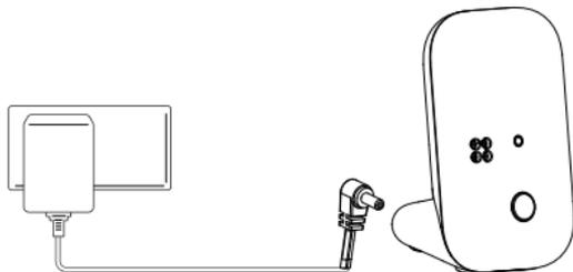
Plug the DC plug of the power adaptor into the DC jack on the rear of the baby unit and plug the other end of the AC adaptor into the AC power outlet.
