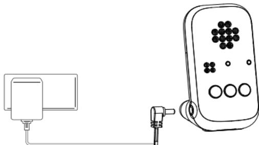
Plug the DC plug of the power adaptor into the DC jack on the side of the parent unit and plug the other end of the AC adaptor into the AC power outlet.
