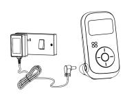
· Insert the DC plug of the power adapter into the DC jack on the side of the parent unit.
